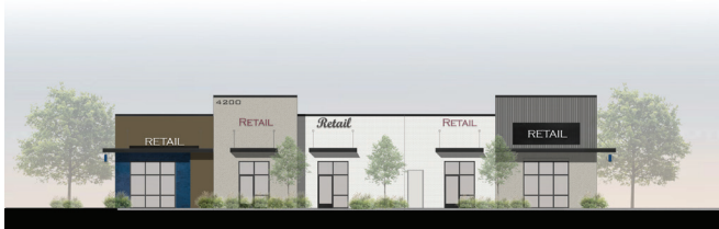
Conceptual Street Elevation Option A: Limited Storefront & Glass Doors with white spandrel or obscured glass
